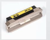
Precision ground prismatic base. Two holes for personal adaptations and brackets.
