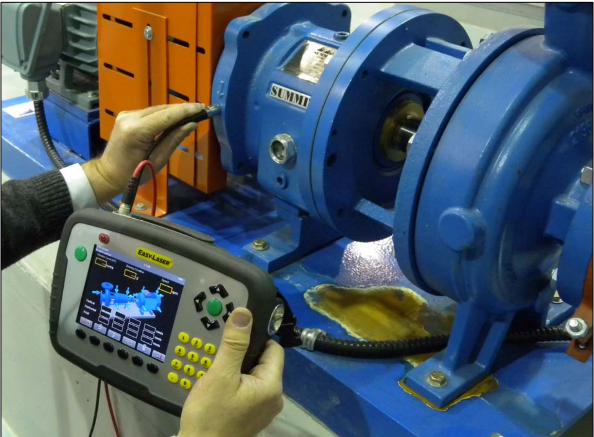
New wireless E-series shaft alignment system, using vibration program as part of the machines PM
