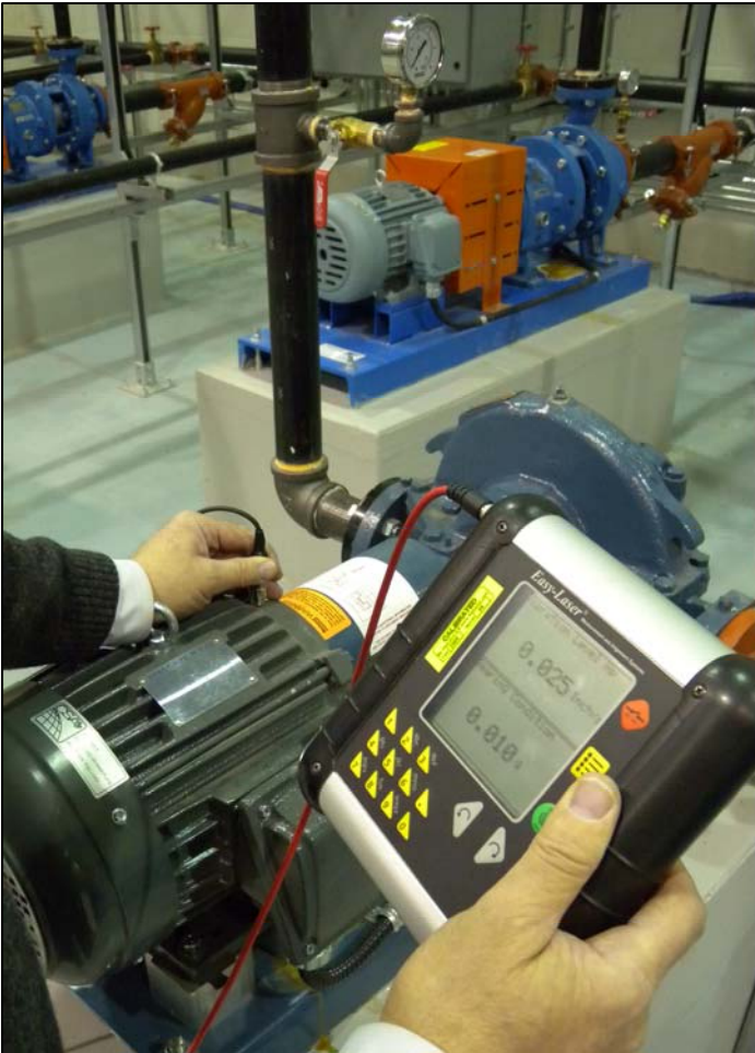
D505 Easy-Laser shaft alignment system using vibration to confirm shaft alignment results.
