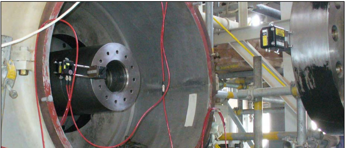
Alignment of a non-rotating shaft.
