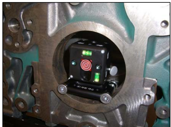
Crankshaft bearing journal measurement of a small diesel engine.
